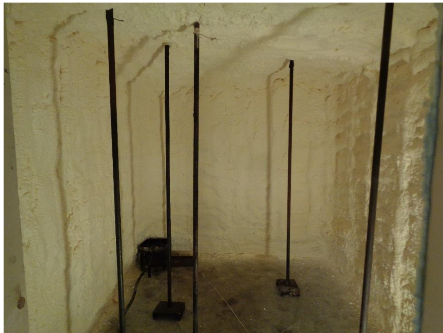
Photo No. 4 Thermocouple and Burner Placement
